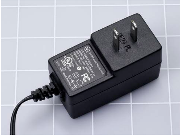
Figure 3-2 An AC adapter that delivers a fixed 9-volt DC output.
