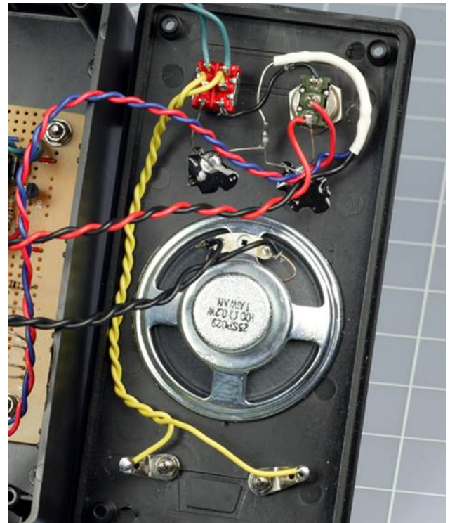
Figure 4-58 Twisted wire pairs have been connected on a point-to-point basis, without much concern over neatness, as this is a relatively small project.
