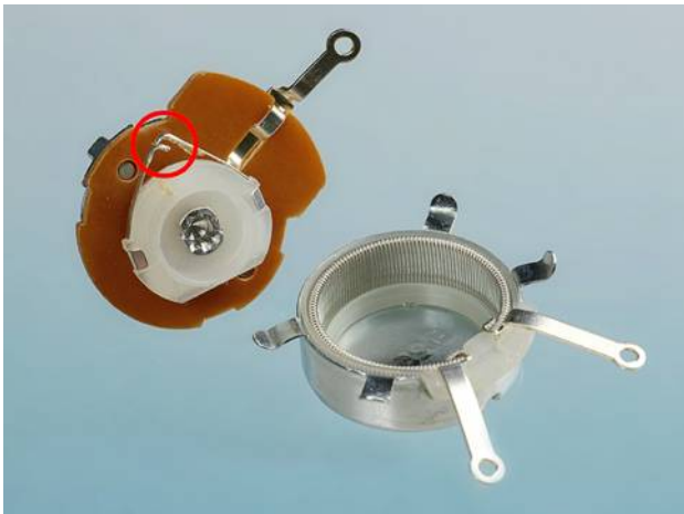
Figure 1-50 The wiper of the potentiometer is circled.
