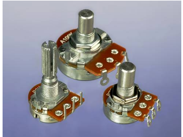
Figure 1-11 Potentiometers of the general type required for your first experiments.
