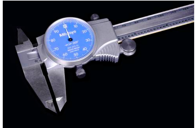
Figure 3-17 Calipers can measure internal and external diameters.
