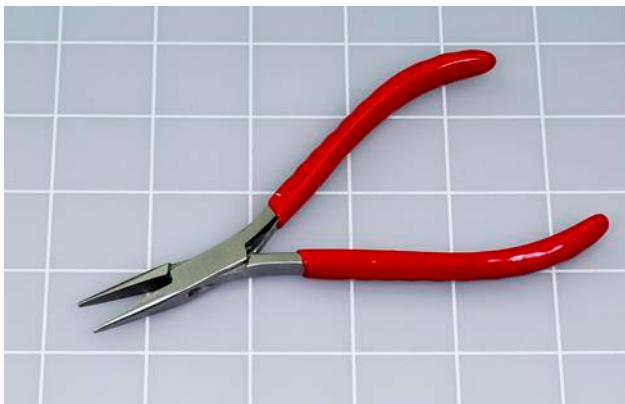
Figure 2-3 Sharp-nosed pliers enable very precise work on a small scale.
