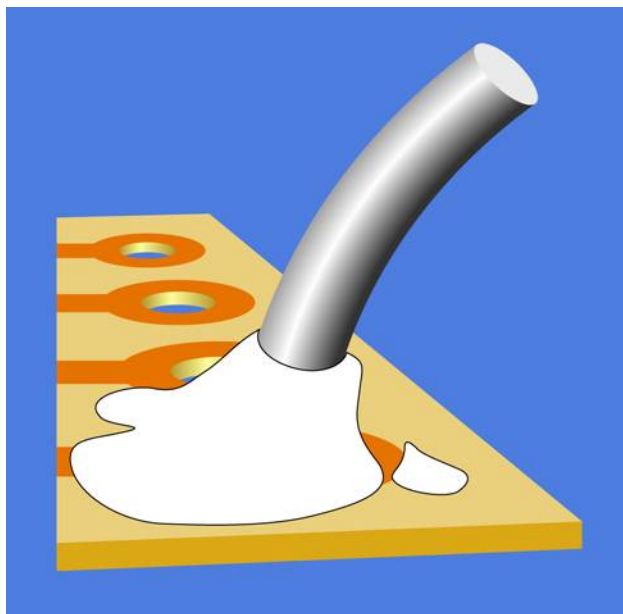
Figure 4-53 If you use too much solder, it will tend to end up in places where you don't want it.
