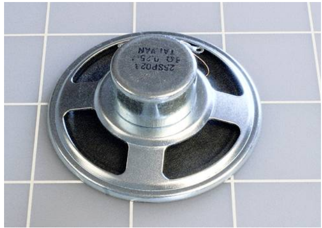
Figure 5-25 The back of a small loudspeaker.
