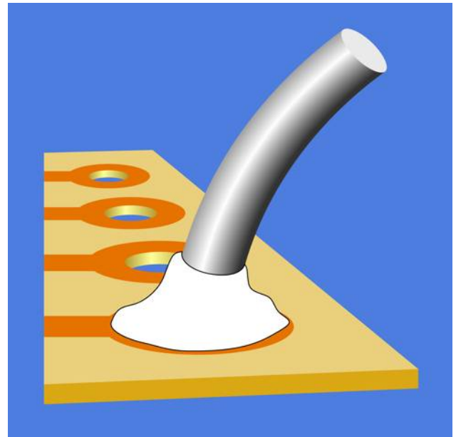
Figure 4-49 Ideally, your solder joint should look something like this.
