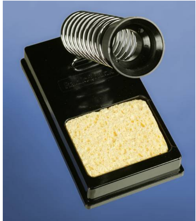
Figure 3-14 A safe and simple stand for a hot soldering iron. The yellow sponge can be wetted with water to clean the tip of the iron.
