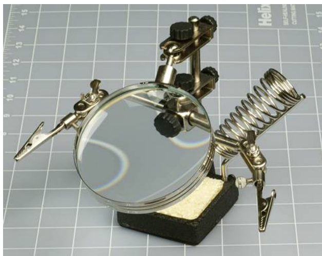
Figure 3-5 The Helping Hand, with additional accessories.
