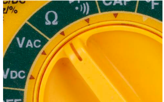
Figure 1-22 On an autoranging meter, just turn the dial to the ohm (omega) symbol.
