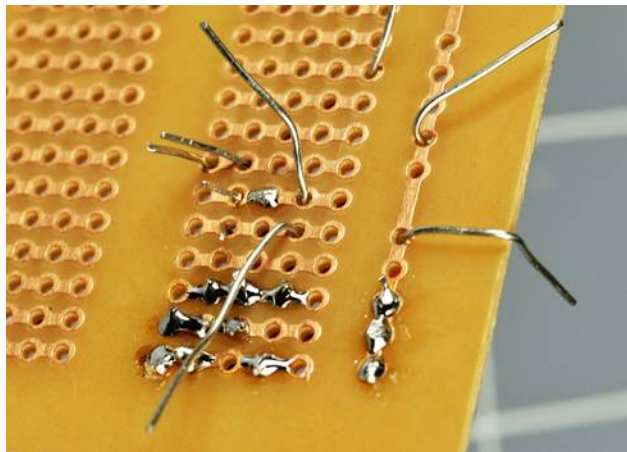
Figure 4-51 This photograph was taken during the process of transferring components from breadboard to perforated board. Two or three components at a time are inserted from the other side of the board, and their leads are bent over to prevent them from falling out.
