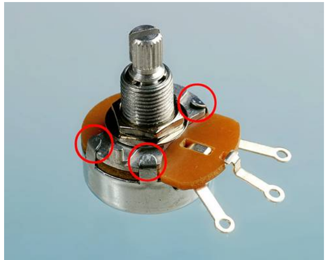
Figure 1-48 The tabs that hold a potentiometer together.
