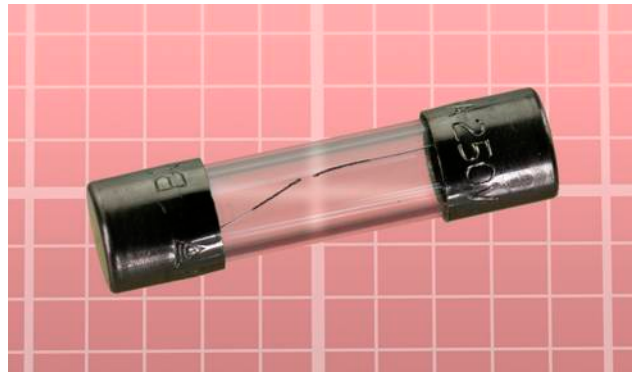
Figure 1-38 In a shorted cartridge fuse, a similar break appears.
