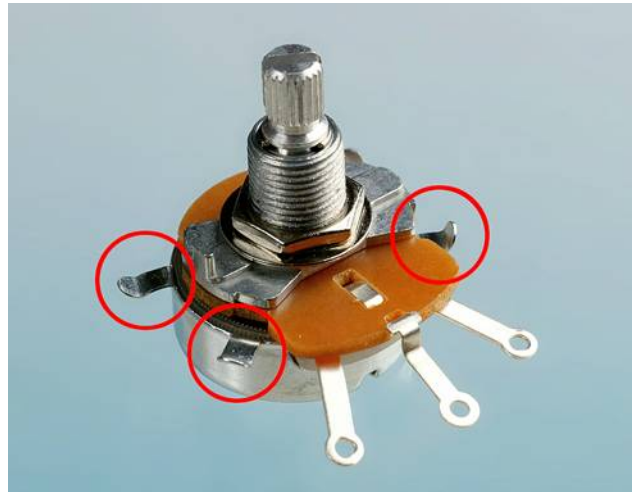
Figure 1-49 The tabs have been bent upward and outward.
