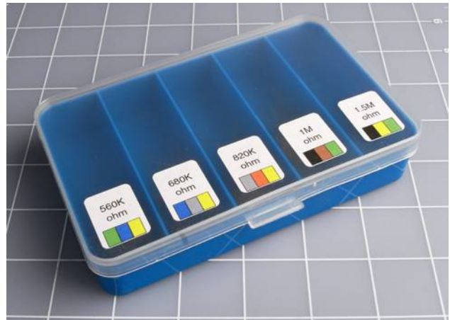
Figure 5-5 To check that resistors are not placed in the wrong compartments, print the color code on each label.
