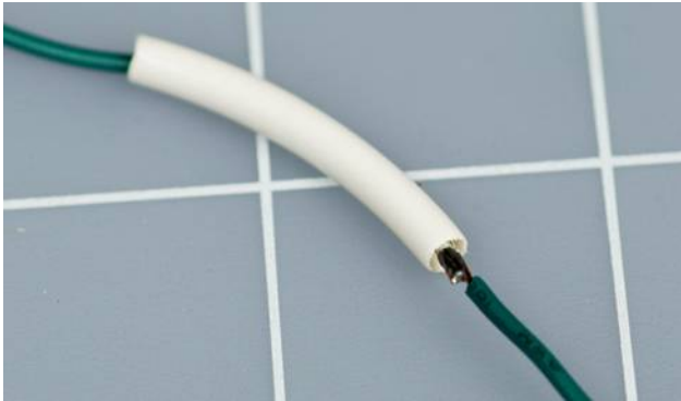
Figure 3-41 Slip the tubing over your wire joint.
