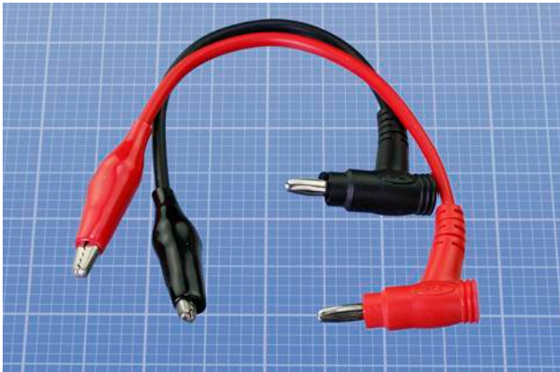
Figure 3-9 Meter leads that terminate in miniature alligator clips.
