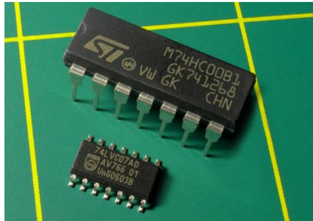
Figure 4-2 A through-hole chip (top) and surface-mount chip (bottom).
