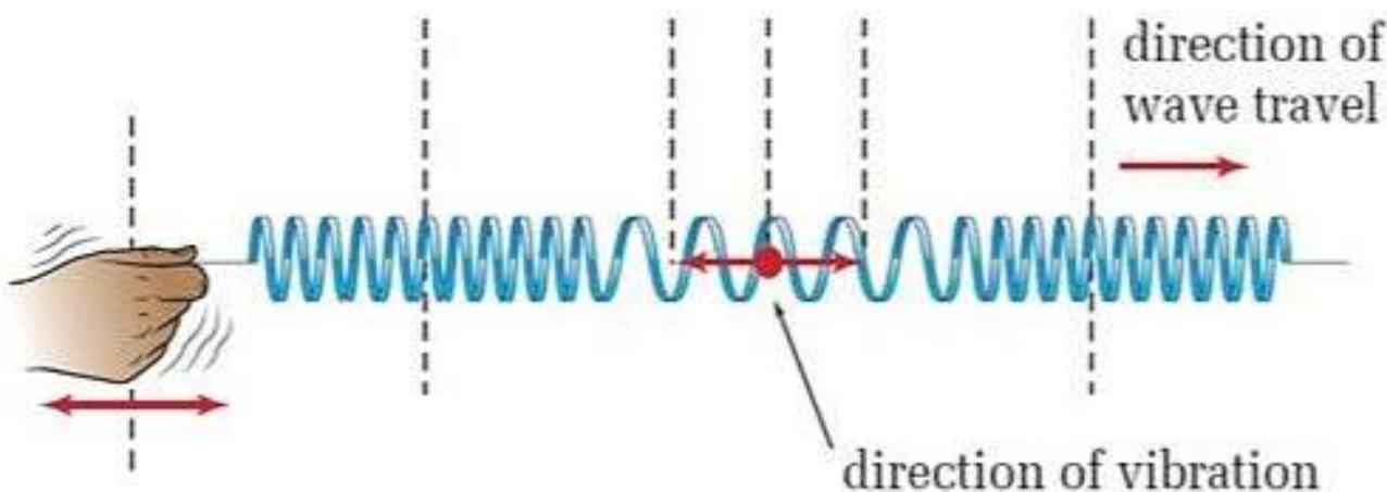
$$\text{Lambda (wave-length)} = \frac{c}{f} = \frac{300}{[\text{MHz}]}$$
